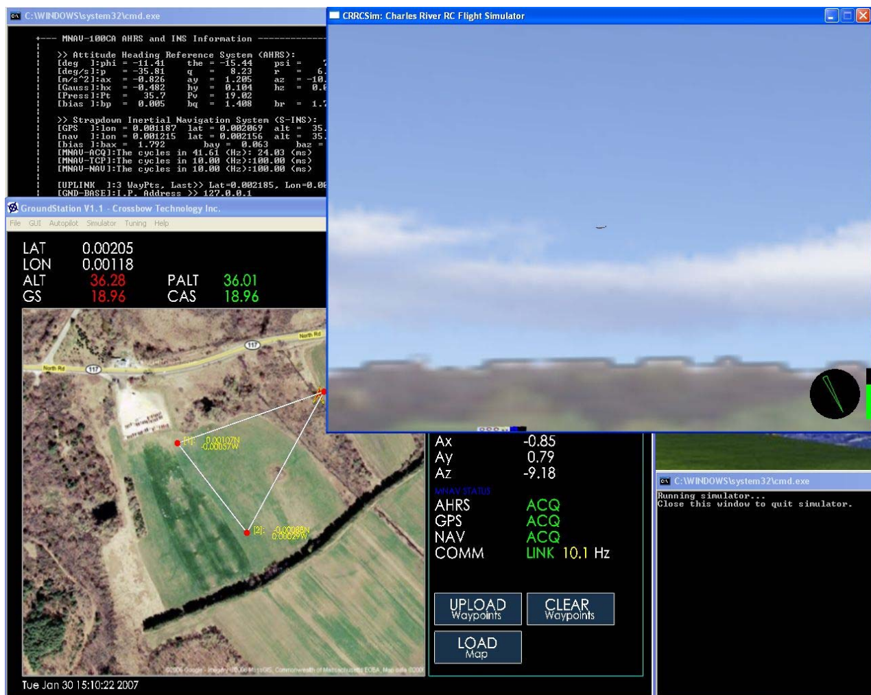
Figure 3: A screenshot of the modified CRRCSim simulator running on the same desktop computer as the MNAV autopilot ground station system. The ZAGI aircraft can be seen in the distance above the clouds in the upper right window, and as the red and yellow swept-wing shape near the upper right waypoint in the ground station viewer.
